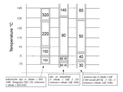
The oil must be of good quality and from the same manufacturer. It is necessary to pour the so-called gear oil.
